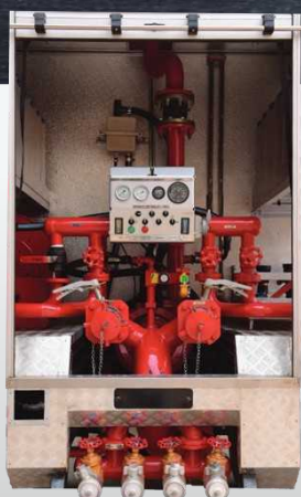
Full Access Control Panel with all controls ergonomically accessible [Optionally Pneumatic Actuated Controls]
